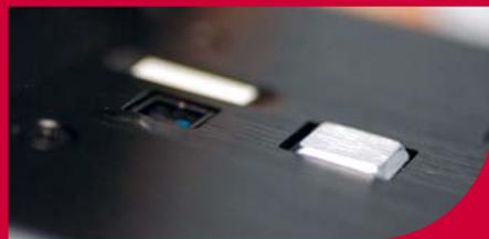
Self-cleaning magnetic sensors keep the device working accurately, even during intensive use. Can be powered with the power cable, batteries, or a 12v adaptor.
