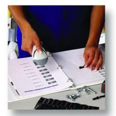
field than a typical CCD. The width of the scan line grows as the scanner moves further away from bar codes. In addition, the laser beam pulses which make lining up bar codes easy, and when the scanner senses a bar code (CodeSense™ Mode), the laser beam automatically switches to scan mode and activates CodeGate to ensure high-speed scanning and accuracy.
