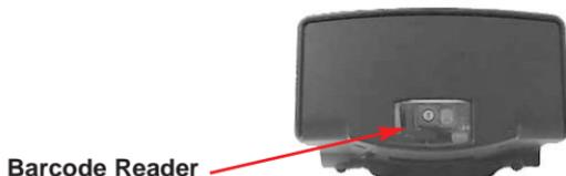
The effective reading distance of the PP-55 barcode reader is approximately 10 cm. To scan a barcode, position the read head as close to the barcode label as possible. Activate the scanner then slowly pull back the unit increasing the distance between the barcode and read head until the barcode has been read by the scanner.
